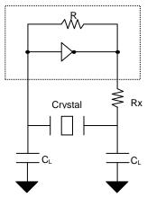
$$\begin{split} C_L &= 2^*(C_P - C_S), \\ Where \ C_P &= Load \ capacitance \ of \ crystal \\ C_S &= Stray \ capacitance \ due \ to \ C_{IN}, \ PCB, \ Trace \ etc. \end{split}$$
